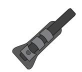
Step 7. Insert pole into bracket.
