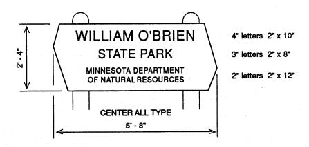
Class A signs are to be installed at large facilities where high visibility is important and in situations of high usage.
